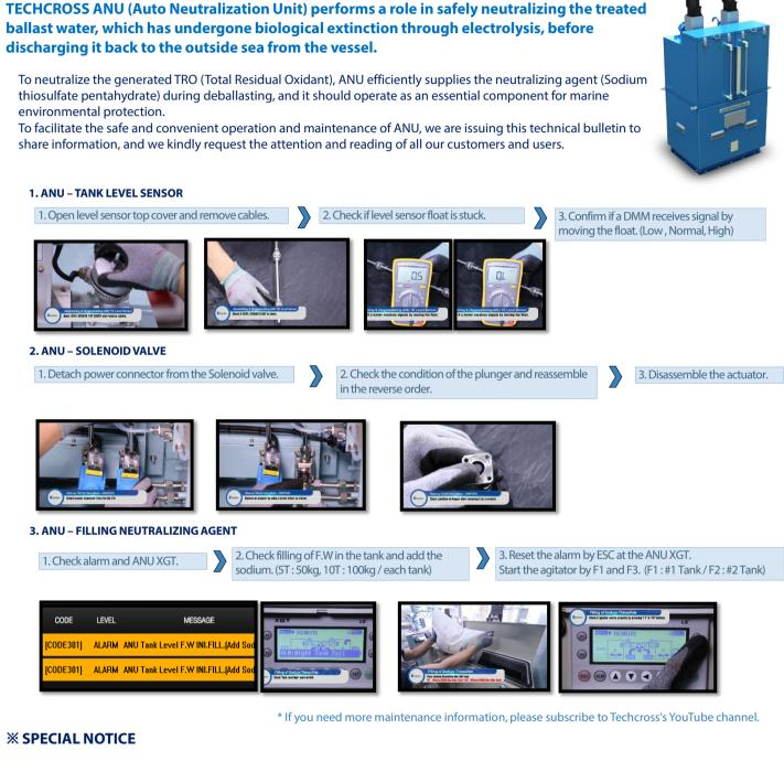
In recent maintenance-related issues at ANU, there has been an increase in case reports of internal corrosion at ANU and cases where proper neutralization is not occurring, due to the use of substandard neutralizing agent.
